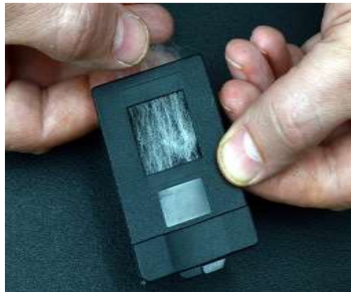
Figure 4: Close sample holder to secure sample
