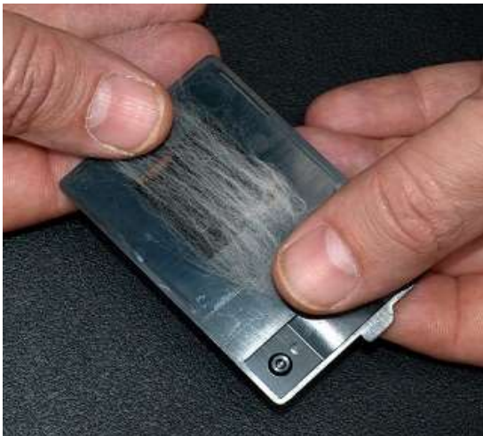
Figure 3: Placing combed sample on sample holder
