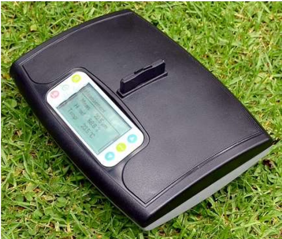
Figure 8: Prepared sample inserted completely in slot on top of FibreLux Meter
